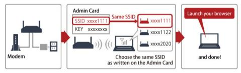
Setting up the router is simple and quick with the web-based setup wizard. First, connect your router and modem, then plug in the router to the AC adapter to turn it on. Secondly, search for the available LAN connection on the network from your computer. Choose the same SSID as written on the Admin Card. Third, launch your web browser and setting screen appears. Set the operation condition as needed to complete the setup. (some environments may require PPPoE settings). It's that simple!
