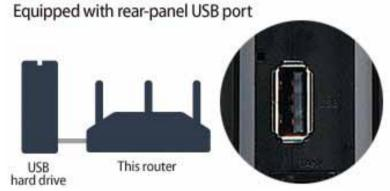
The router is equipped with a USB port that lets you connect a USB hard drive, USB flash memory, or other USB storage devices. You can connect a USB drive and use it as a networked attached storage (NAS) for sharing data from your home PC or digital appliances. There are no complicated settings to make—just connect the USB cable to turn your USB hard drive into an additional NAS.
